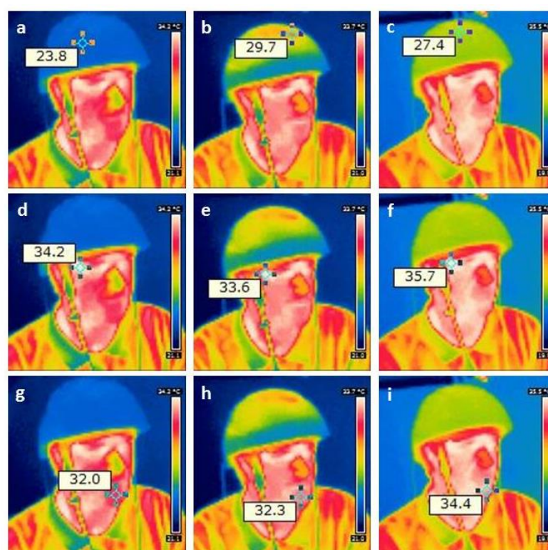
Figure 4. Results from thermal imaging of the first pilot measurement using the new stimulation helmet. Note the increase in temperature on the helmet (upper row; a before, b during, and c after stimulation) on the forehead (middle row; d – f) and on the chin (lower row; g – i).
